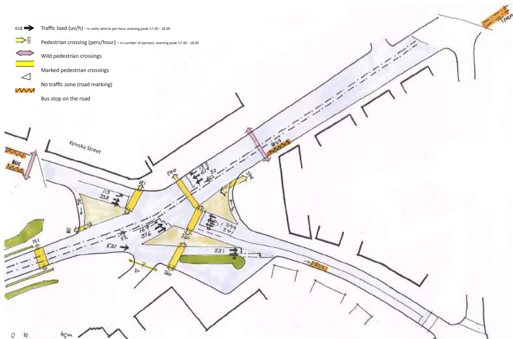
Figure: Junction on Zhovtneva Square, current geometry, pedestrians crossings and traffic load 17:30 – 18:30
